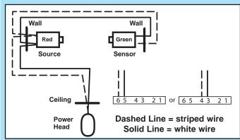
FIG. 4-5b Pre-Wired source and sensor wiring methods.
